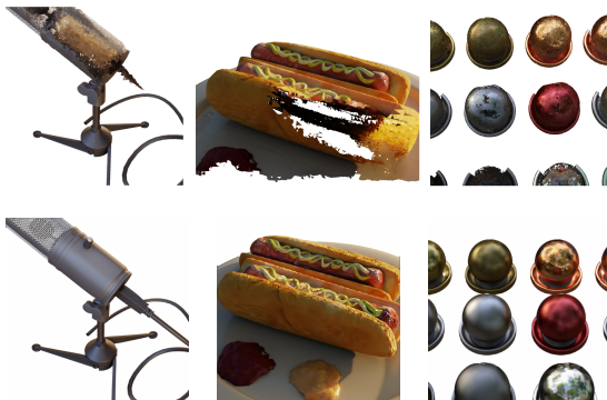
Figure: Zoom-in comparisons. Top row : MobileNeRF (Chen et al., 2023). Results are obtained from the code and demo released by the authors. Bottom row : MobileR2L. Our approach renders high-quality images even for zoom-in views.
